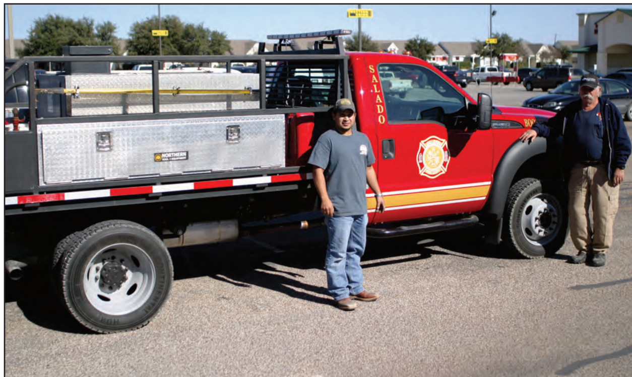
Salado Volunteer Fire Department members Lt. A J Lopez (left) and Chief Charles Young (right) brought this up-graded fire truck by the Salado Village Voice office for a short tour. The fire fighting unit was moved to a 2013 model truck chassis to increase the service life of the unit. PHOTO BY TIM FLEISCHER
