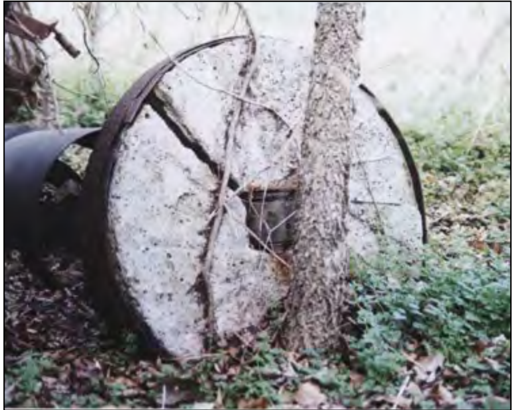
Ike Jones Mill millstone with gears and pulley with attachment to a drive belt to power machinery. (Photograph courtesy of Dr. David J. Mikulencak.)
