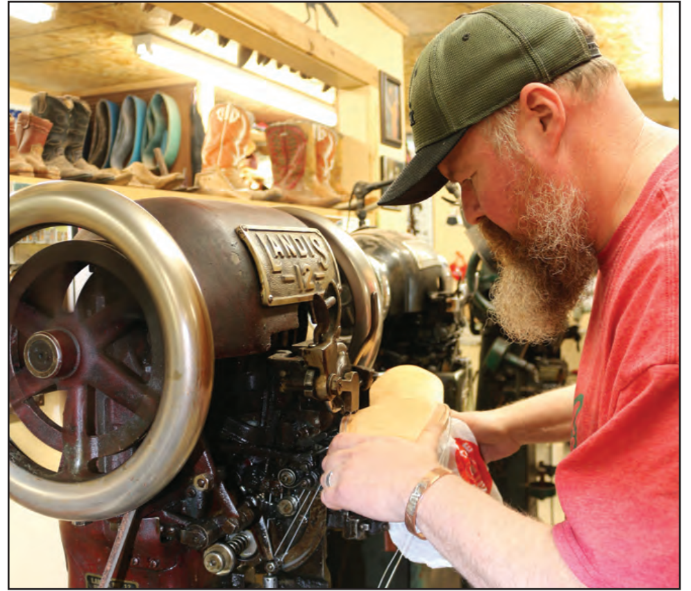
Dustin Lauw attaches the sole of a custom cowboy boot using a vintage Landis 12 sole stitcher at his Salado shop, Duck's Heritage Cowboy Boots. PHOTO BY STEPHANIE HOOD
