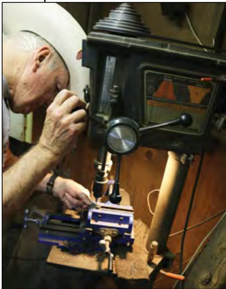
Bill Smith puts a divot on a blade so that it will snap into place. (Photo by Tim Fleischer)
